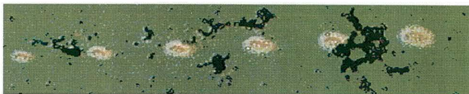
Figure 5.23 Optical microscope image of a PCDM film showing the effect of laser exposure (light, circular areas) and polymer aggregations (irregular, dark areas).
