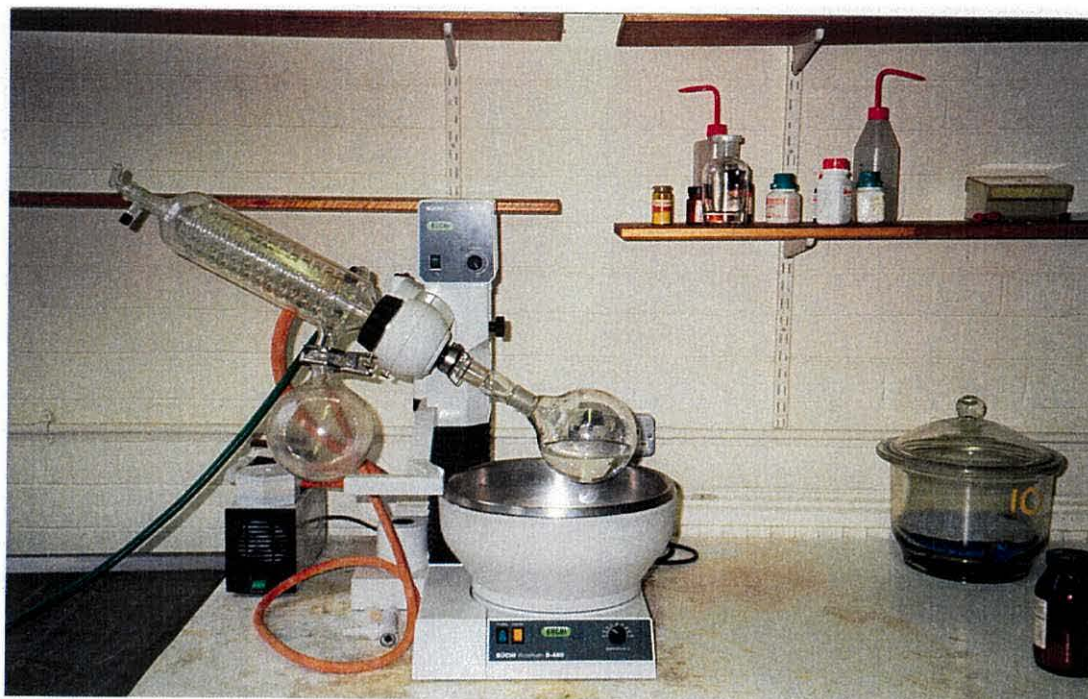
Plate 4.2. Rotary evaporator used to evaporate the solvent to get the oil
