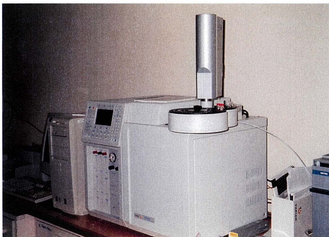
Plate 4.3 GS apparatus/machine used in santalol identification and determination of the amount contained in the oil
