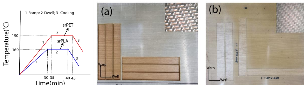
Figure 1 Typical cure cycle employed to fabricate srPET and srPLA laminates. Photographs of the (a) srPET and (b) srPLA woven fabric and cured composite laminates.
