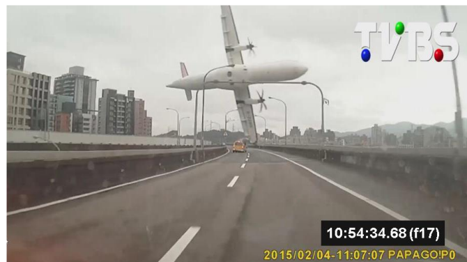
Figure 1. Snapshot of the dashboard camera video which was used in the investigation of Flight GE235 to synchronise CVR time, flight path, and aircraft attitude (Aviation Safety Council, 2016).
