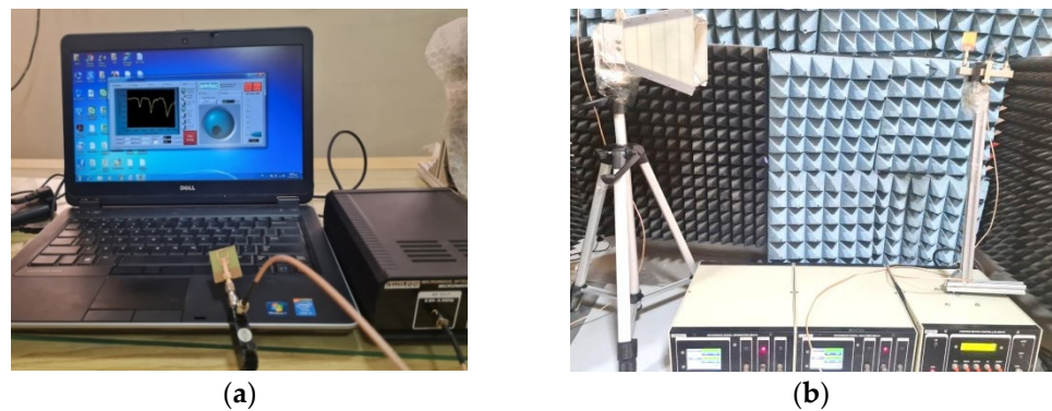
Figure 10. The measurement setup of (a) the reflection coefficient curve and (b) the radiation pattern and gain.
