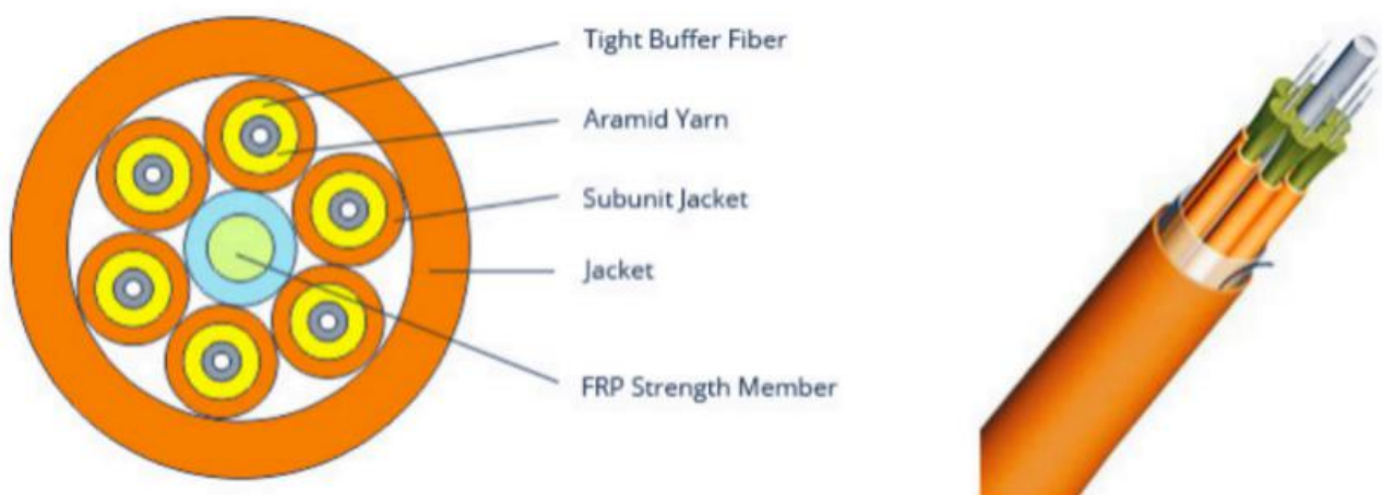
Fig. 5 Breakout Fiber Optical Fiber
