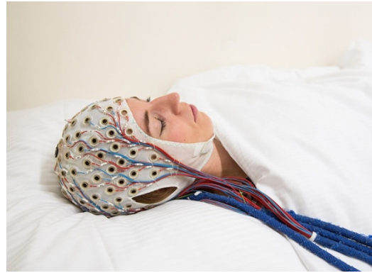
Figure 5: Sleep recording with 128 Electrode Sleep EEG cap.
