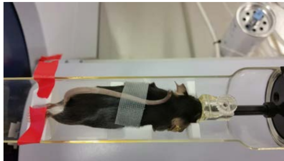
Figure 4.2.: Photograph of a mgr/mgr mouse in a custom made bed for in-vivo \mu\text{CT} . Here, the mouse is positioned into the bed (white plastic). Especially, the feet are taped to a foot bank, which is then repositioned (and fixed with the red tape) stretching the legs for clear and straight CT images, which makes the segmentation much easier. The tail is taped slightly to the fur for the same reason. The mouse is also attached to a tube infusing isoflurane for anaesthesia during the imaging time.
