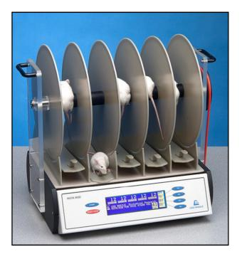
**Fig. M-6: Rotarod (Ugo Basile):** ROTA-ROD for mice; picture modified after the instruction manual of the ROTA-ROD for MICE (Cat. No. 47600), provided by Ugo Basile.
