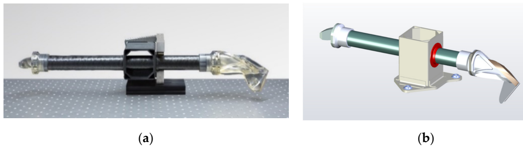
Figure 10. (a) Qualification model of the RRU of the LRI of GRACE-FO; (b) NGGM RRU concept with smaller beam separation and modified mounting interface.
