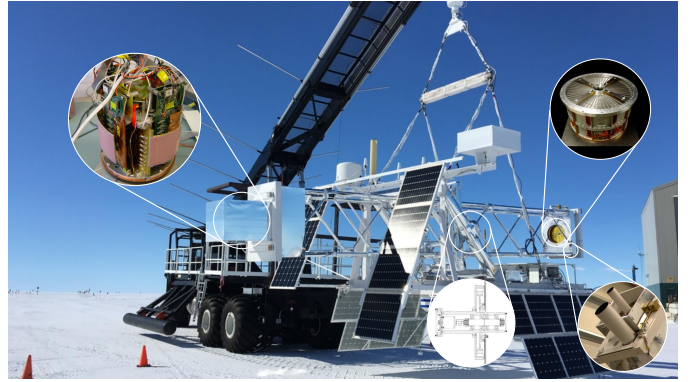
Figure 2: The X-Calibur payload and its main components during the final compatibility test at the McMurdo Long-Duration Balloon Facility. Highlighted from left to right: the X-Calibur polarimeter at the focal point of the X-ray telescope; the WASP torque motors used to point the system; the InFOC \mu S X-ray mirror; the CARDS star tracker.
