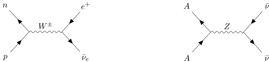
(a) IBD: an electron antineutrino \bar{\nu}_e scatters off a proton, creating a positron and a neutron mediated by a vector boson W^\pm .
