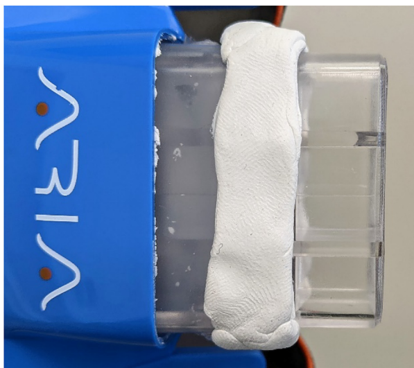
Fig. 7. A) Photo of the soft plastic seal of the mask (extending to yellow intermittent line), black rubber seal, and hard plastic snorkel connector. B) Circumferential putty placement prior to inserting adapter. C) Adapter pushed in as far as possible and covering the soft plastic seal. Putty extruded circumferentially without any gaps to have an airtight and secure connection. (For interpretation of the references to colour in this figure legend, the reader is referred to the web version of this article.)
