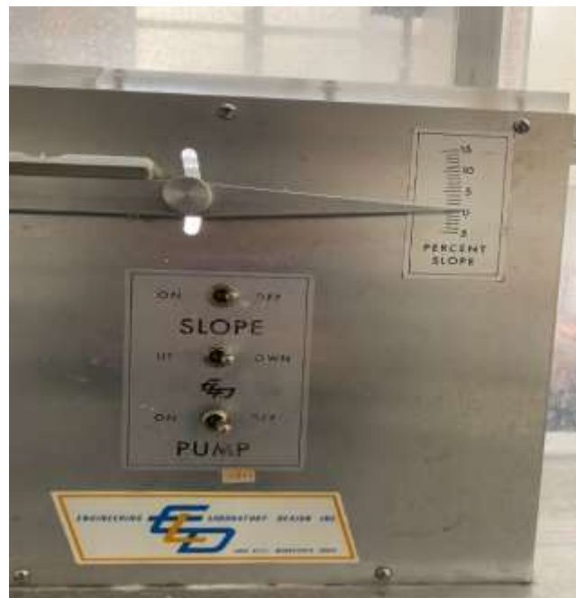
Figure 19. The configuration of the water tunnel and the slope that defines the velocity.
