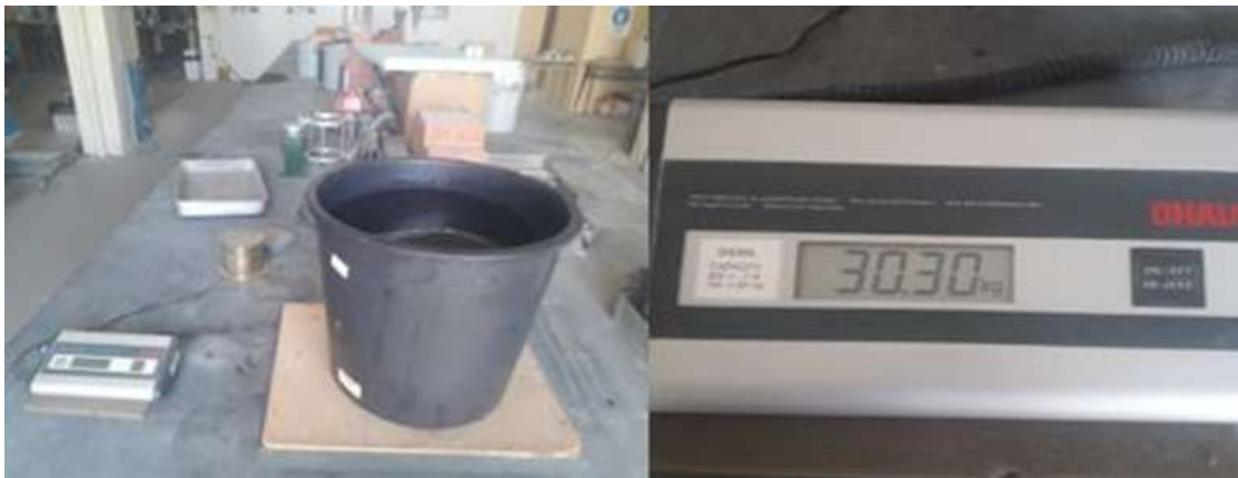
Figure 18. Mass of container with water.
