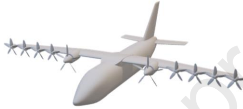
Fig. 9 Hybrid-electric commuter aircraft under development in ELICA framework.
