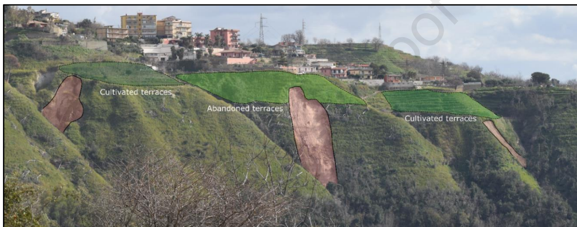
296 297 Figure 4. Interaction between land-use change (green) and landslides (light red). Lateral landslides were detached at the 298 base of the terraced areas where the agricultural practices are still active, differently from the central landslide.
