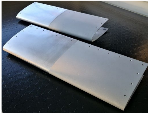
Figure 3. Leading Edge for Lamb-wave test
