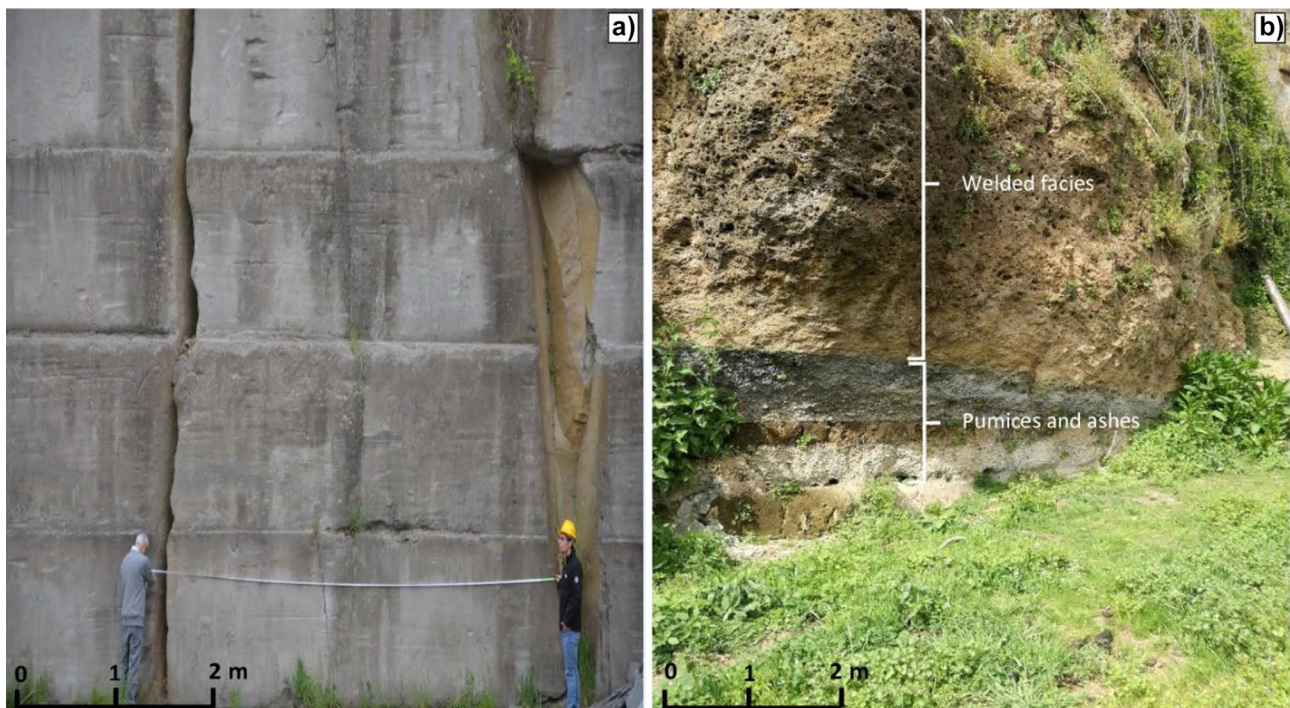
Fig. 2 Examples of ICV (a) and CIV (b) survey outcrops (a horizon of pumices and ashes is visible at the base of the welded facies of the CIV)
