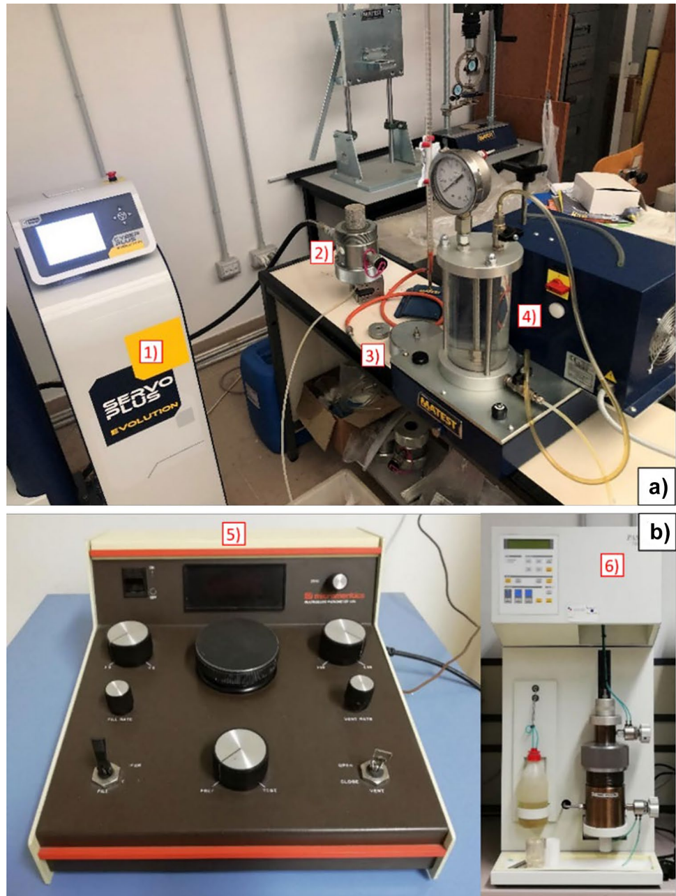
Fig. 4 Laboratory equipment for measurements of hydraulic conductivity (a) and porosity (b). 1) Servo-Plus evolution control unit of the spherical confining pressure; 2) Hoek cell with the specimen; 3) End cap; 4) Oil–water control system of the water back pressure by manometer; 5) MultiVolume Pycnometer 1305; 6) Thermo Finnigan Pascal porosimeter 140
