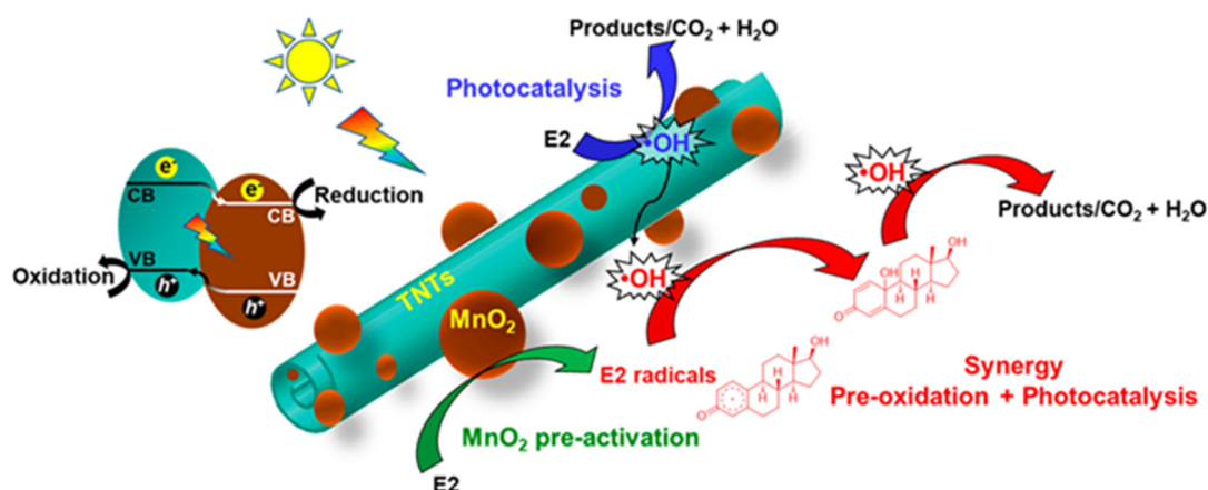
Figure 13. The schematic mechanism of the degradation of E2 by using MnO 2 NPs decorated titanate nanotubes (TNTs). Reprinted with permission from [161], Copyright (2018) American Chemical Society (ACS).
