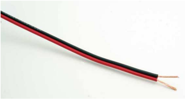
Fig. 1. Picture of the biwire used as sensing element.
