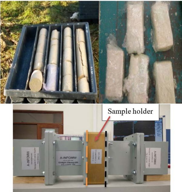
Fig. 2. The samples and measurement setup used to measure the permittivity of GL in the laboratory.
