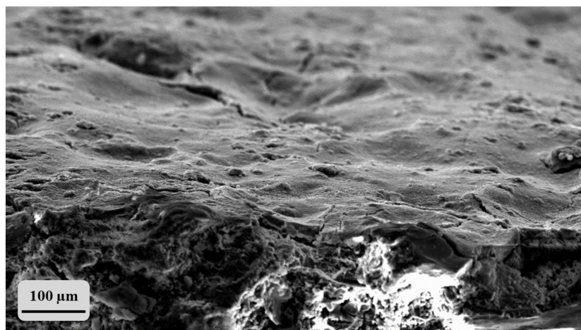
Figure 6. SEM image of CI after brushing treatment with pure LS.
