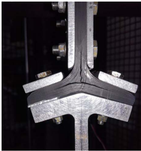
(a) Crack propagation
