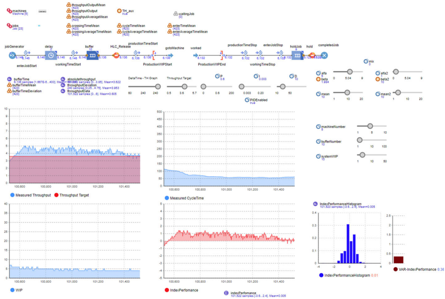
Fig. 11 The control action response to a TH change
