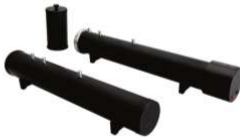
Figure 2: Typical example of Kundt tube.
