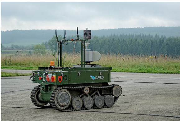
Fig. 5. RMA tEODor UGV with the 3D mapping hardware.
