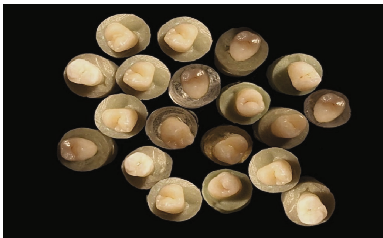
FIGURE 1: Teeth mounted in cylindrical acrylic resin blocks.
