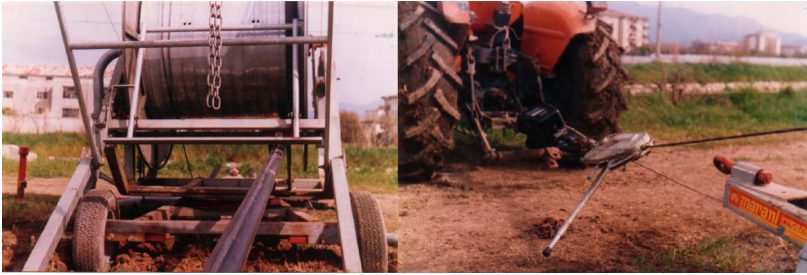
a) Pipeline rewinding phase b) Experimental test to evaluate the pull force
