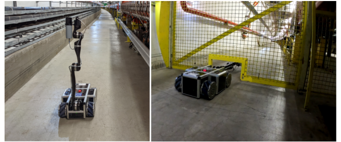
Fig. 1. The MIRA SPS Robot during inspection (left) and the MIRA Robot crossing one of the sector doors (right).
