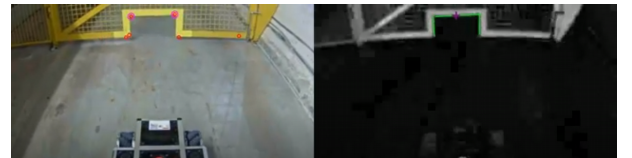
Fig. 9. Contour points (left image) used for the initialization of the segment tracker (right image).
