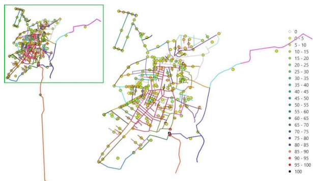
Fig. 6 WDN-Relevance-based betweenness centrality for the segment graph of Real WDN
