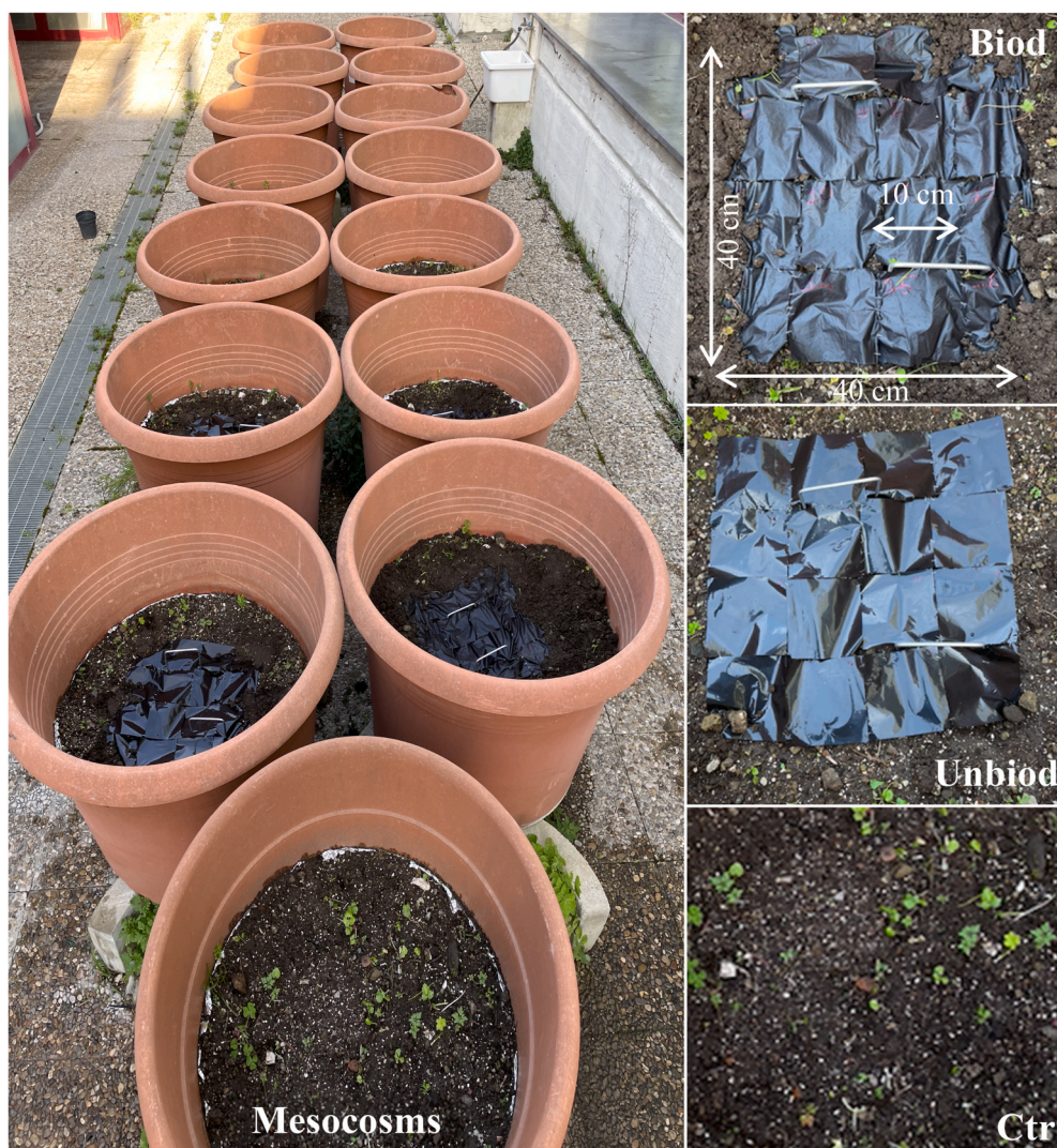
Fig. 1. Experimental mesocosms (left) and details of soils covered by un-biodegradable and biodegradable plastic sheets and uncovered soils (right).
