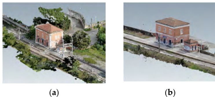
Figure 11. Survey activity results in terms of point clouds (a) for a railway station and (b) for a railway stop.
