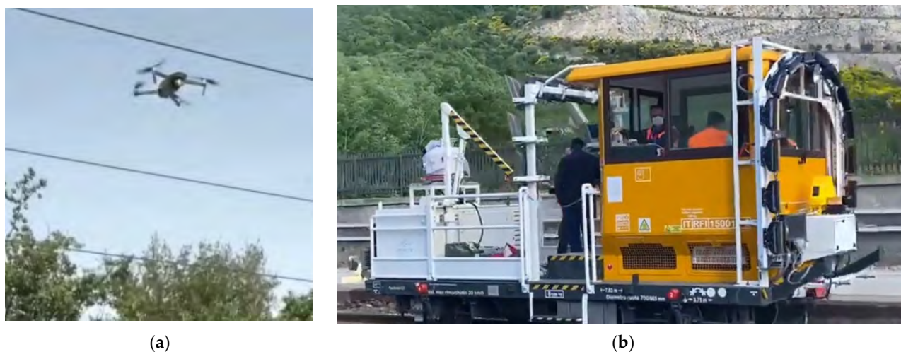
Figure 3. Surveying equipment engaged for existing condition acquisition of railway line: (a) drones; (b) autonomous railway vehicle.
