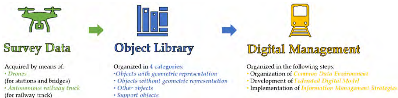
Figure 4. Definition of a digitalization strategy for existing railway infrastructure.
