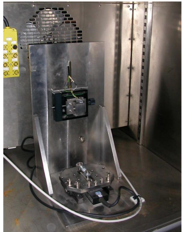
Figure 10: Photograph of the sensor during the zero and sensitivity shift in the PARANI UC 150 climatic chamber
