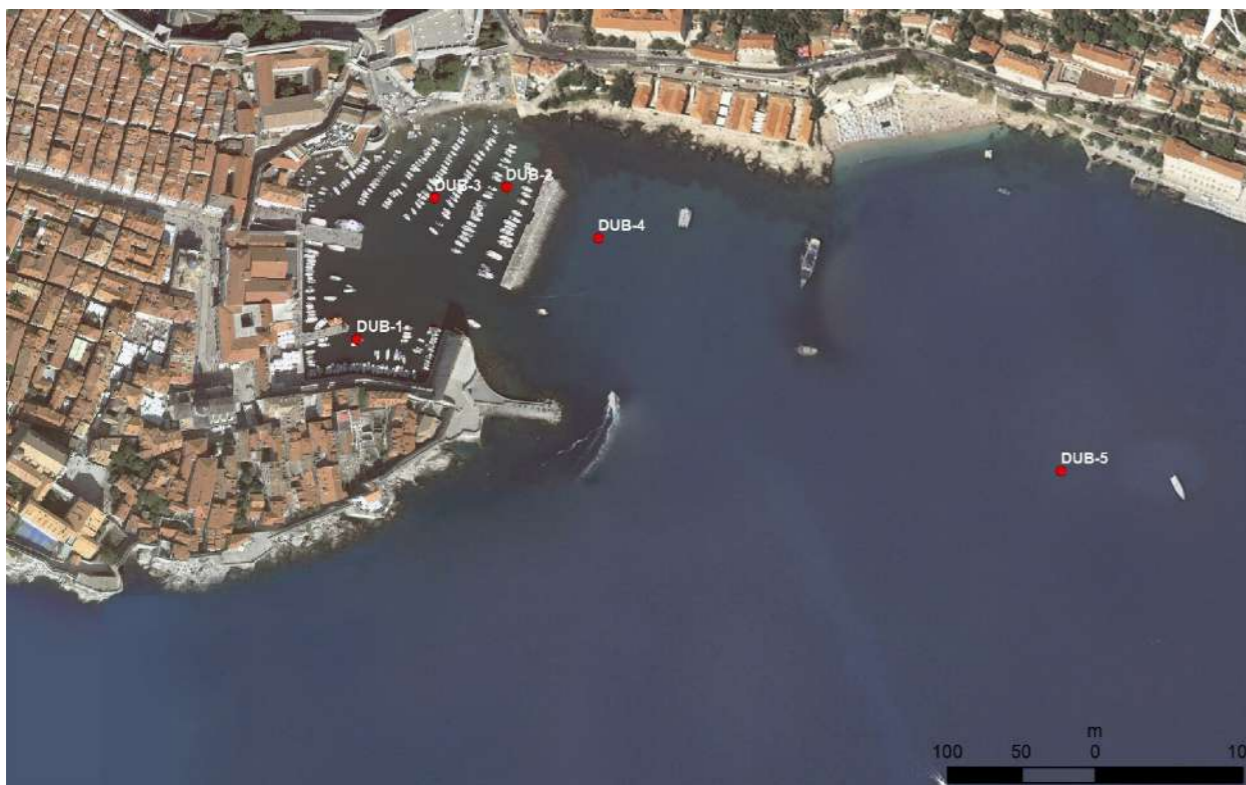
Fig. 24 Positions of geological cores (Croatian Geological Survey)
