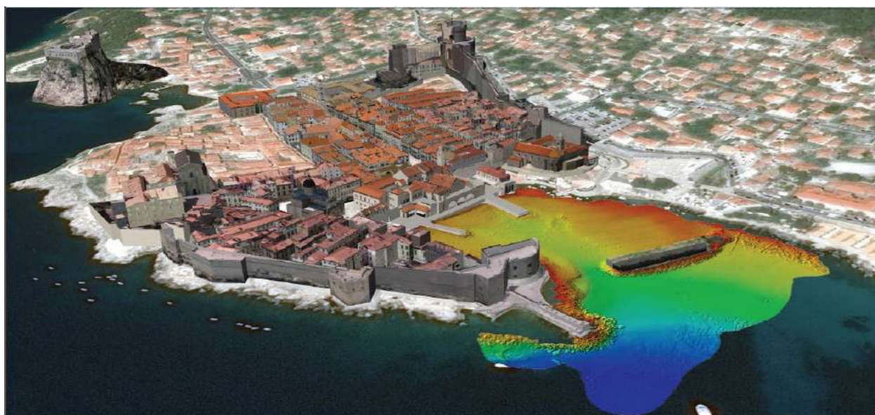
Fig. 17 Digital terrain model opened in Google Earth application (GEOmar Ltd.)
