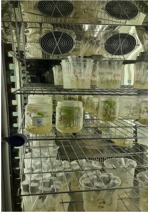
Figure 14. Thermotherapy incubator in the CIP lab for heat treatment of explants before meristem excision.
