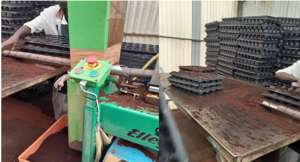
Figure 5. Cocopeat filled in plugs (left) and the plugs fitted into trays (right).
