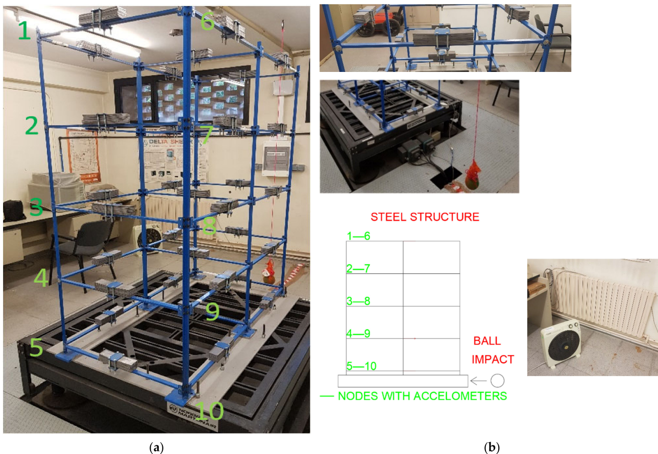
Figure 2. (a) Scaled steel model structure with the number nodes (green); (b) The added load, the ball, schema representing the structure, the monitored nodes (green), and the heaters.
