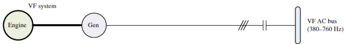
Fig. 5 VS VF power generation scheme Source: [14]
