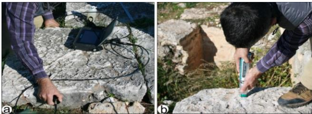
Figure 7. Sonic velocity and Schmidt Hammer tests applied on rocky ground (Tağa & Güler, 2018)
