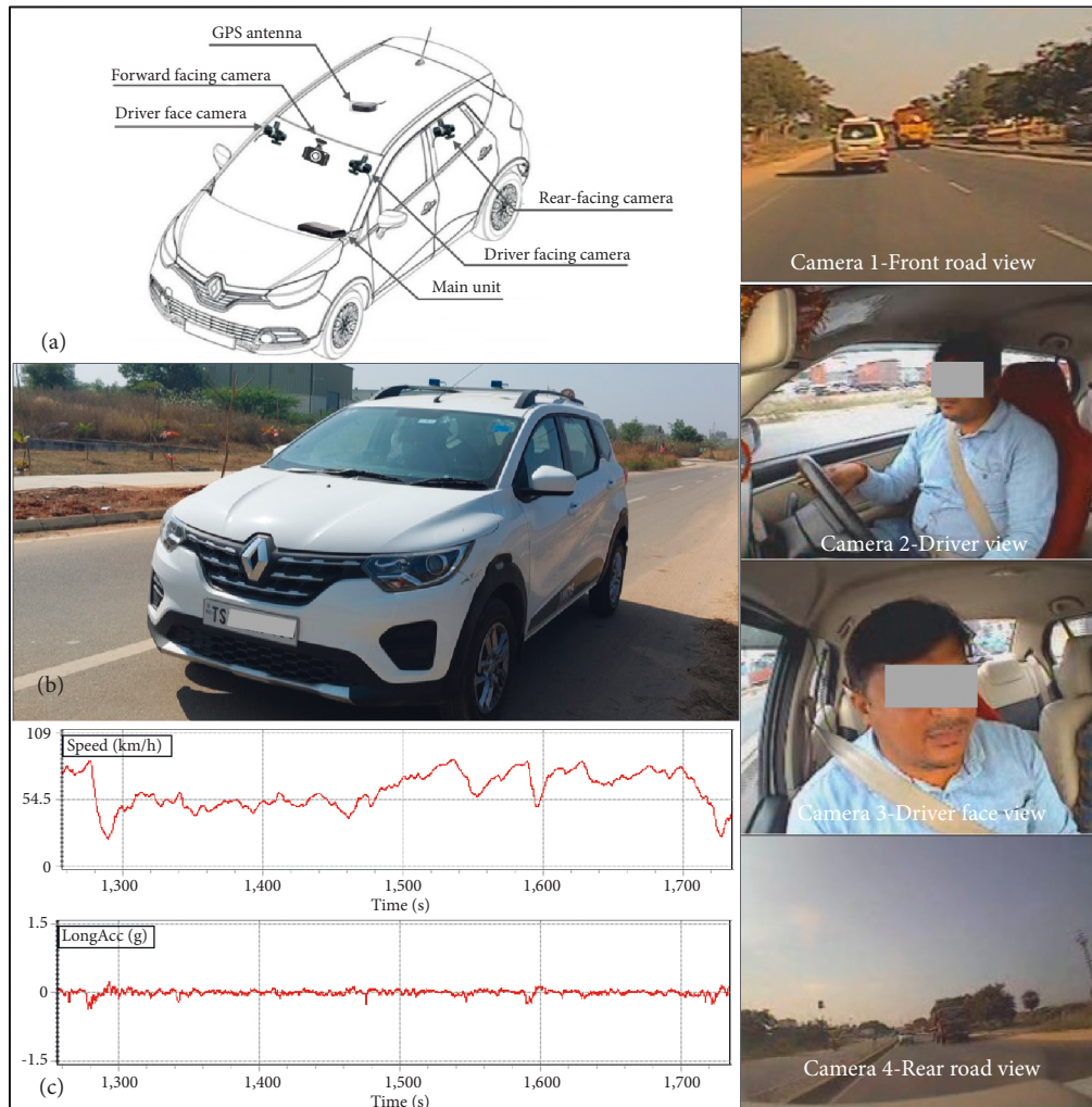
FIGURE 2: (a) Instrumentation details; (b) Study vehicle; (c) Recorded speed and acceleration profiles; and snapshots of collected video data.
