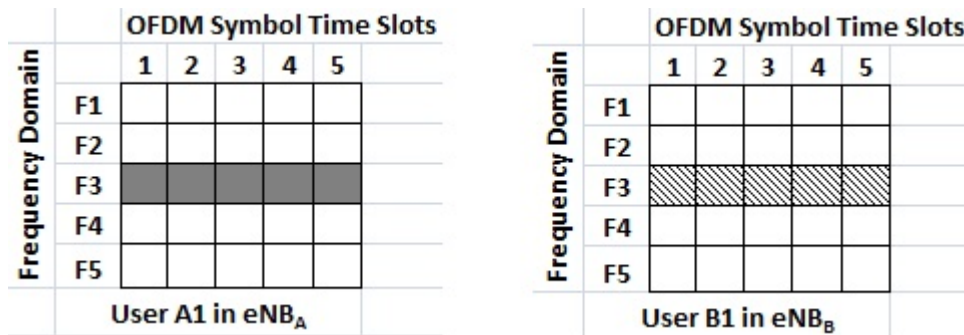
Figure 30. An example of the worst case resource allocation for one user per eNB.
