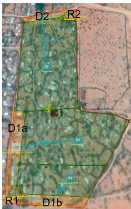
Figure 9a – Layout of the SRCDS D1a, D1b, D2 and reservoirs (R1 & R2)
