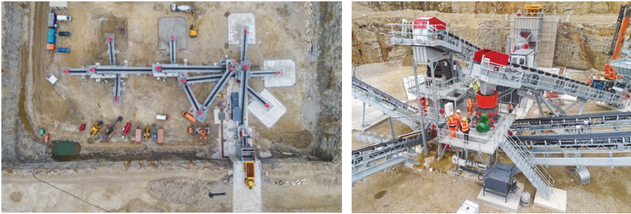
Figure 1.5 Typical C&S plant from above, and a side view of the secondary station in the plant.
