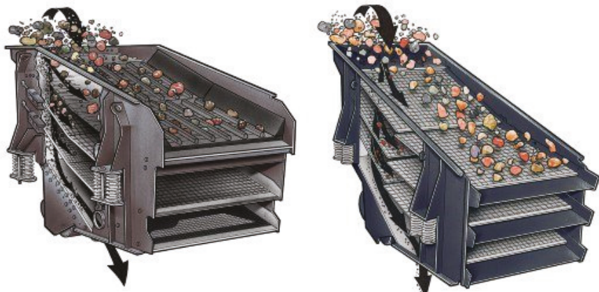
Figure 1.10 The two main screening principles: right, screening through stratification, and left, screening through free-falling [4].
