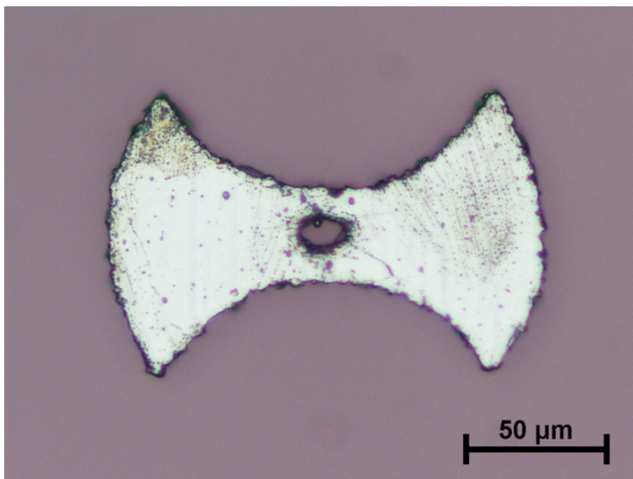
Figure 2.17: Photomicrograph of a rhenium IRH filament drilled with three overlapping holes to create an oval sample chamber. This allows the sample chamber to take a more circular shape as it deforms at high pressure.
