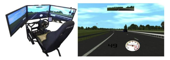
*Note*. The left panel shows the driving simulator with the tablet device positioned next to the steering wheel. The right panel shows the central monitor view of the driving environment with rear-view mirror and digital speedometer displayed.<sup>1</sup>
