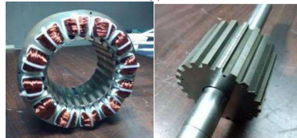
Fig. 35. The hybrid-excited structure with RMSS PM [103]. (a) Topology. (b) Prototype.
