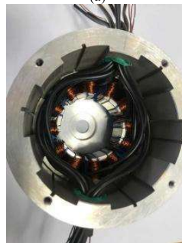
Fig. 17. The TMSS-PM DSM with modular topology [62]. (a) Topology. (b) Prototype.
