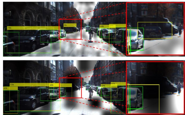
Fig. 2. Detections in the distorted image with IoU: (top) minimum obstruction kernel size l = 12 \times 12 pixels (bottom) minimum obstruction kernel size l = 72 \times 72 pixels.
