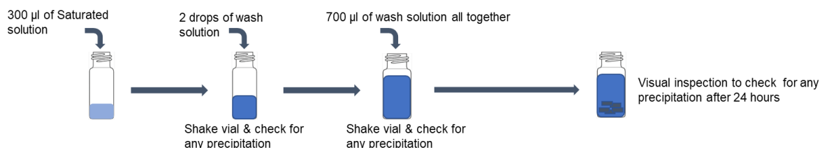
Figure 1: Glass vial precipitation detection method.
