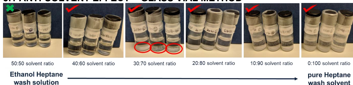
Figure 3: Ethanol - n-heptane glass vial precipitation qualitative test.
