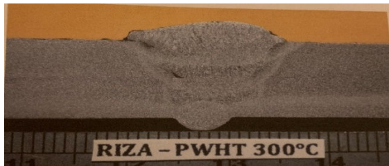
Figure 9. Macrostructure of specimen with 300°C post heating temperature
