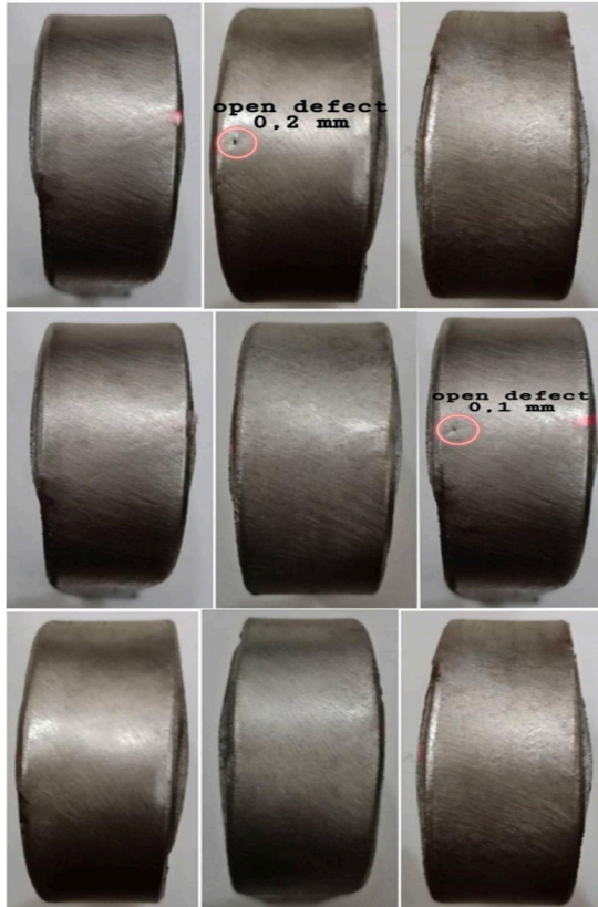
Figure 12. Visual Pictures of The Result of Bending Test of 3 PWHT Varieties
