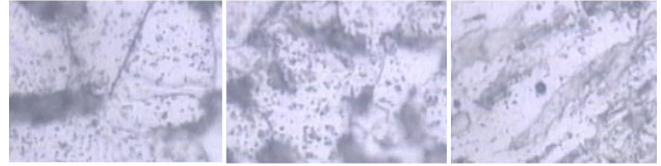
Figure 6. Microstructure of specimen with 350°C post heating temperature
