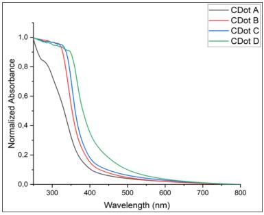
**Figure 3.** The results of UV-Vis spectra from CDots samples with varying concentrations of 5% (CDots A), 10% (CDots B), 15% (CDots C), and 20% m/v (CDots D)
