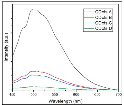
Figure 5. Results of PL spectra of CDots samples with varying concentrations of 5% (CDots A), 10% (CDots B), 15% (CDots C), and 20% m/v (CDots D)
