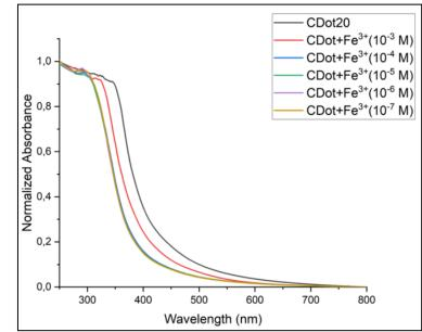
**Figure 4.** The results of the UV-Vis spectra of the Fe<sup>3+</sup> metal ion detection sample with variations in concentrations of 10<sup>-7</sup>, 10<sup>-6</sup>, 10<sup>-5</sup>, 10<sup>-4</sup>, and 10<sup>-3</sup> M
