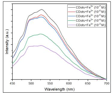
**Figure 6.** The results of the PL spectra of the heavy metal ion detection samples of Fe3+ with variations of 10<sup>-7</sup>, 10<sup>-6</sup>, 10<sup>-5</sup>, 10<sup>-4</sup>, and 10<sup>-3</sup> M
