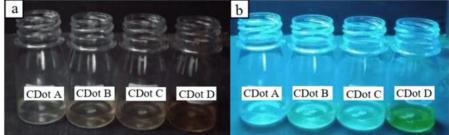
Figure 1. CDots sample (a) without UV lamp, (b) exposed to UV lamp
