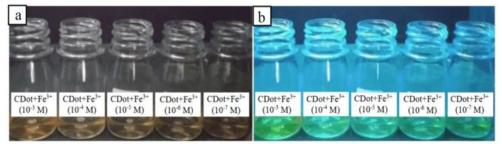
Figure 2. Sample CDots+ $Fe^{3+}$  (a) without UV lamp, (b) exposed to UV lamp
