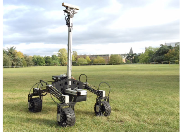
Fig. 6. The robotic platform used for experiments. The robot is a commercially-available version of a planetary rover. It is equipped with low-power motors, a stereo camera pair for visual localisation and a CPU to carry out the computation.
